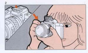
Press the shutter release button all the way down to trip the shutter and activate the flash.
