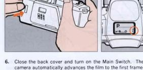
Close the back cover and turn on the Main Switch. The camera automatically advances the film to the first frame. Make sure that the LCD panel displays the [ / ] and **Q\_\_\_O** ] indications.
